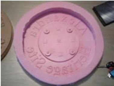
Mould cast and tested
